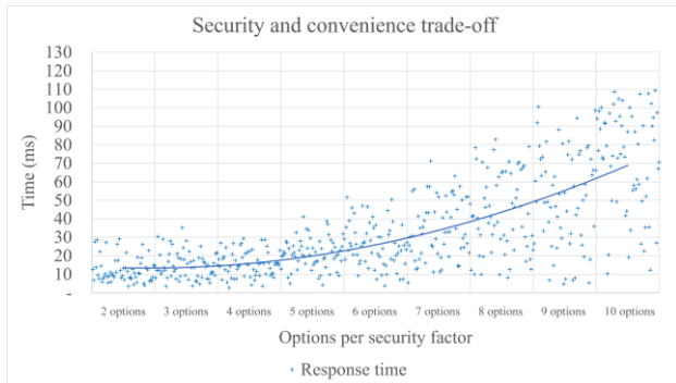
Figure 3. The results obtained in Task 2, in which we investigated the trade-off between security (i.e., the number of available options for each digits) and convenience (i.e., time required to verify the PIN). The chart shows users' response times.
